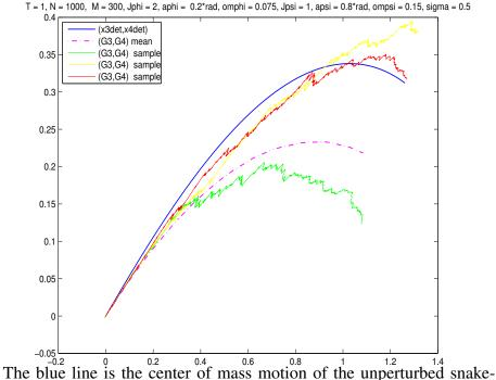
The blue line is the center of mass motion of the unperturbed snakeboard and the dotted magenta line is the mean motion of the stochastic snakeboard with the same deterministic input. Additionally 3 sample plots have been included. The data are as indicated above: T is the runtime, 1/N the step size, M the number of experiments, rad  $=\frac{180}{\pi}$  and  $\sigma$  the parameter specifying the strength of the white noise. The initial conditions are  $q_0=(0,0,0,0,0.5)$ .
