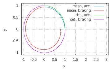
The data are  $\rho=1$ ,  $D_1=1.2$ ,  $D_2=0.8$ , R=0.3, c=0.1. we have plotted the accelerating and braking parts of  $(E[x_t], E[y_t])$  as blue and red, and the accelerating and braking parts of the unperturbed controlled robot (x(t), y(t)) as green and magenta, respectively.
