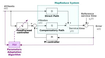
Fig. 1. MapReduce model and control schema
