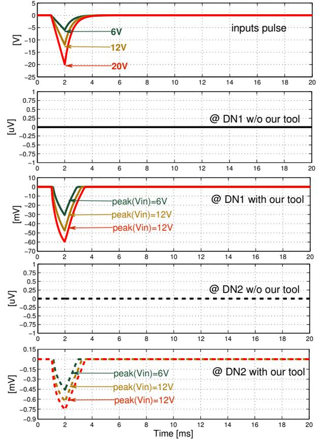
Fig. 15. Result of fast transient simulation with automotive test pulse: as 6V, 12V or 20V peak voltage. Voltages simulated at output on  $50\Omega$  with or without our tool. Laser cut option to choose the corresponding N-well: DN1 or DN2.
