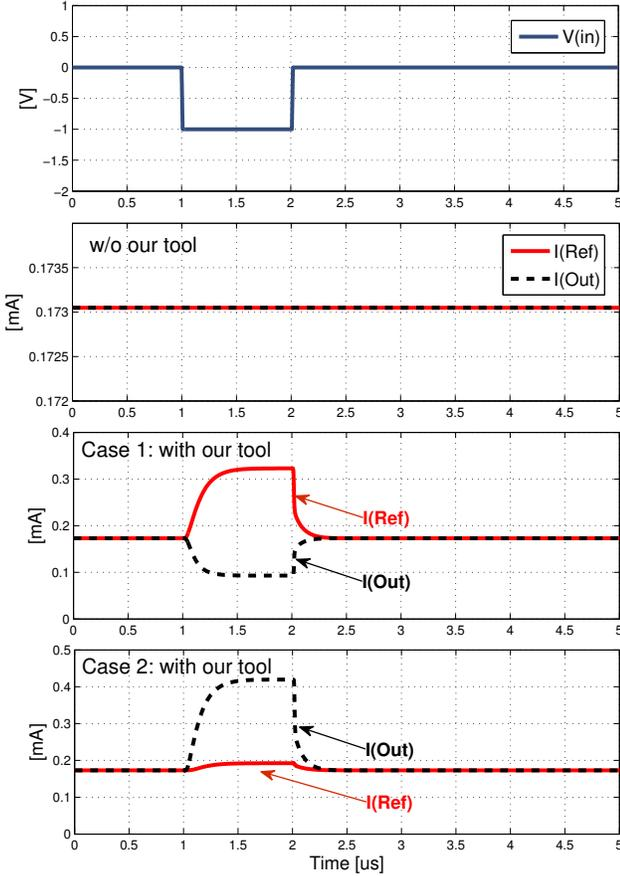
Fig. 13. Transient behaviors with substrate current injection.
