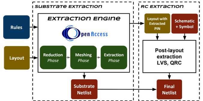
Fig. 2. Overall flow of post-layout extraction.
