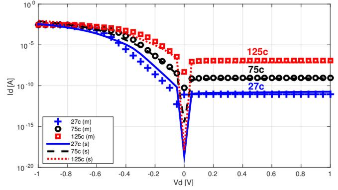
Fig. 6. Temperature behaviors in both forward and reverse biased conditions, at 27°C (blue), 75°C (black) and 125°C (red).
