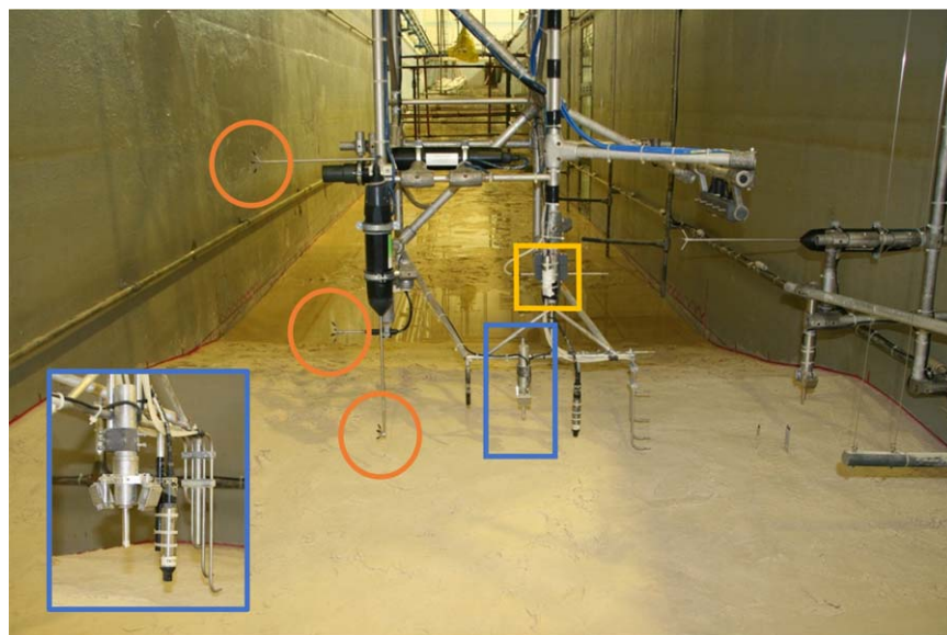
Figure 2. Photo of measuring frame, taken from top of breaker bar while facing the beach. Highlighted instruments: ADVs (orange circles); PT (yellow square); and ACVP (blue rectangle). Inset shows close-up of ACVP.
