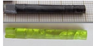
FIG. 2: Picture of the single crystal, as grown (top) and annealed (bottom) used in the present study.
