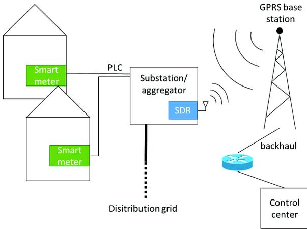
Fig. 1. Communications of the advanced metering infrastructure
