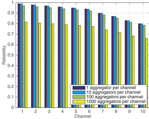
Fig. 5. Reliability of the AMI backhaul in each channel versus the number of aggregators in the channel
