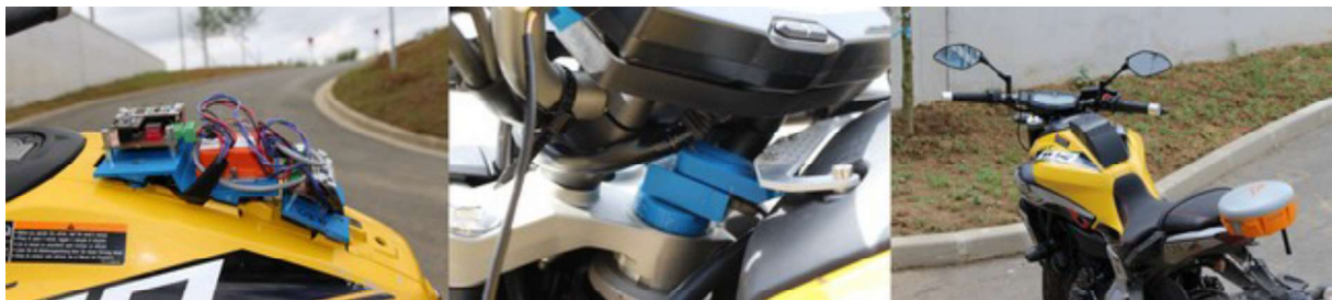
Picture 2. the MT07 with some sensors: IMUs, steering wheel, RTK-GPS
