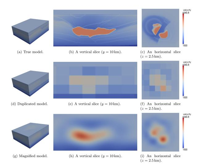
Figure 5: 3D duplicated and magnified models of the SEG/EAGE salt dome velocity model. The velocity models are built using  $n = 8 \times 8 \times 5 = 320$  parameters, while  $N = 225 \times 225 \times 70 = 3543750$  parameters are required for the true velocity model.
