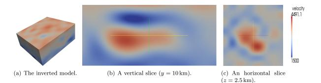
Figure 7: Inversion results for the salt dome velocity model using n = 320 parameters. The 1 Hz case.
