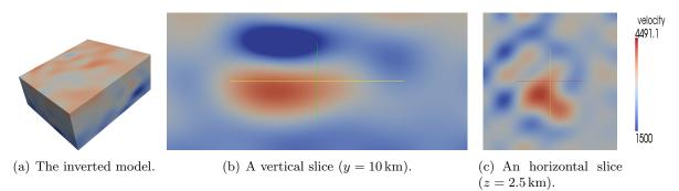
Figure 8: Inversion results for the salt dome velocity model using n = 320 parameters. The 2 Hz case.
