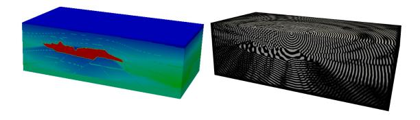
Figure 2: 3D SEG/EAGE salt dome velocity model: problem geometry with velocity distribution (left) and real part of numerical solution at 12 Hz (right). Figures from [26, Chapter 4].
