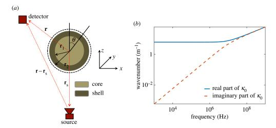
**Figure 1.** (a) Cross section of the core—shell structure used for studying the scattering of DPDWs. (b) Dispersion relation in the background medium, region 0: Real and imaginary parts of  $\kappa_0$  versus frequency. (Online version in colour.)
