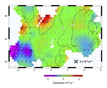
**Figure 8.** Smoothed horizontal strain rate field for the Western Alps and Pyrenees region. Dashed lines are strain rate standard error. Light grey curves show the drainage pattern and dark grey curves the seashores and country borders.
