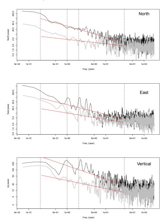
**Figure 5.** Noise spectra for site MTPL. Spectra derived form the unfiltered time series are in black, those for the filtered time series are in grey. The red lines represent the best spectral models used for the uncertainty analyses.
