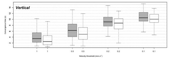
**Figure 4.** Whisker plots of convergence time for four velocity thresholds  $(1.0, 0.5, 0.2, \text{ and } 0.1 \text{ mm yr}^{-1})$ . Thick bars, boxes, and dashed bars represent the median, quartile (25 and 75 %) and extreme values of the distributions for the 44 stations with at least 10 years of data. Grey and white whisker plots correspond to unfiltered (raw) and filtered (with common-mode correction) data.
