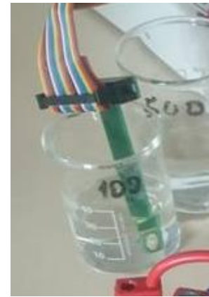
Figure 2: Part of the measurement setup involving immersion of the probe in different samples of calibrated conductivity standards.
