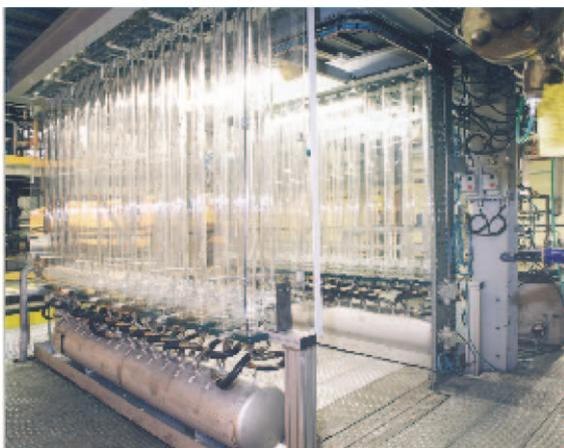
Fig. 26. Gas-liquid separator system associated to the collector tray.
