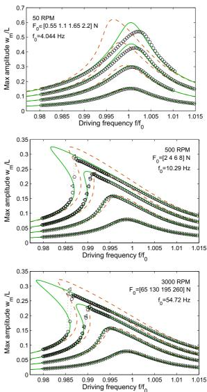
**Fig. 6** First bending mode frequency response for various rotation velocities and various forcing amplitudes  $F_0$ . Maximal amplitude of tip oscillations normalized by beam length  $(w_m/L)$  as a function of driving frequency normalized by the natural fre-
