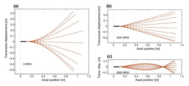
**Fig. 5** Large amplitude oscillations of the beam at resonance, FE model. **a** Mode 1, no rotation (0 RPM), largest forcing of Fig. 6; **b** mode 1, rotation at 3000 RPM, largest forcing of Fig. 6; and **c** mode 2, rotation at 3000 RPM, largest forcing of Fig. 7
