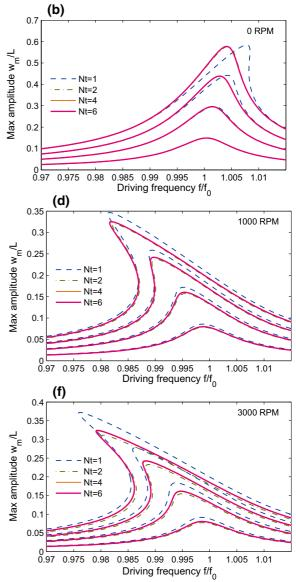
*Right column* (**b**,**d**,**f**): same curves as a function of the driving frequency normalized by the natural frequency of the mode computed with  $N_t$  transverse modes
