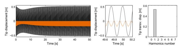
Fig. 4 Time evolution of the tip of the beam at mode 1 resonance, FE model, rotation at 3000 RPM, transverse and axial displacements. Zoom in the steady state. Fourier series decomposition of the transverse displacement in the steady state
