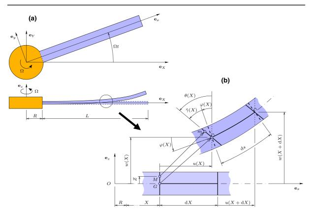
Fig. 1 a Sketch of the rotating beam. b Detail of a beam element deformation
