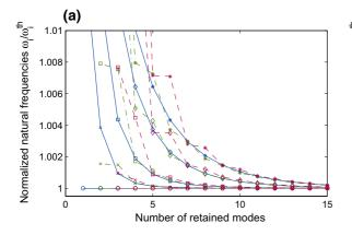
Fig. 3 Convergence of the natural frequencies as a function of discretization and rotation velocity. Normalized natural frequencies  $\omega_i/\omega_i$ th, where  $\omega_i$ th is the numerical value at full resolution of the model (20 modes for the analytical models and 200 elements for the FE model). **a** VK and Inxt models (identical
