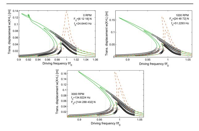
Fig. 7 Second bending mode frequency response for various rotation velocities and various forcing amplitudes  $F_0$ . Maximal amplitude of tip oscillations normalized by beam length  $(w_m/L)$  as a function of driving frequency normalized by the natural fre-
