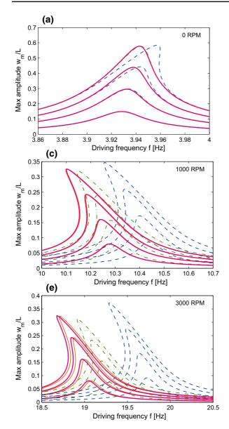
Fig. 9 Convergence of the Inxt model, around the resonance of the first bending mode, as a function of the number of transverse modes  $N_t$  retained in the expansion of Eq. (66). *Left column* (**a**,**c**,**e**): resonance curves as a function of the driving frequency.
