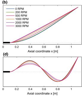
Fig. 2 Linear modes dependence upon the rotation velocity (FE model with 200 finite elements). **a** Natural frequencies of the four first modes as a function of  $\Omega$ ; **b**,**c**,**d** deformed shapes of the
