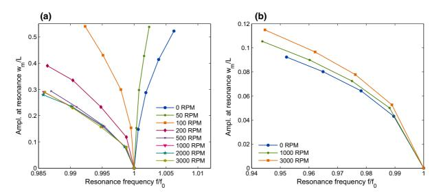
Fig. 8 Backbone curves of **a** mode 1 and **b** mode 2. Normalized resonance amplitude as a function of normalized resonance frequency (FE model) for various rotation velocities and various forcing amplitudes
