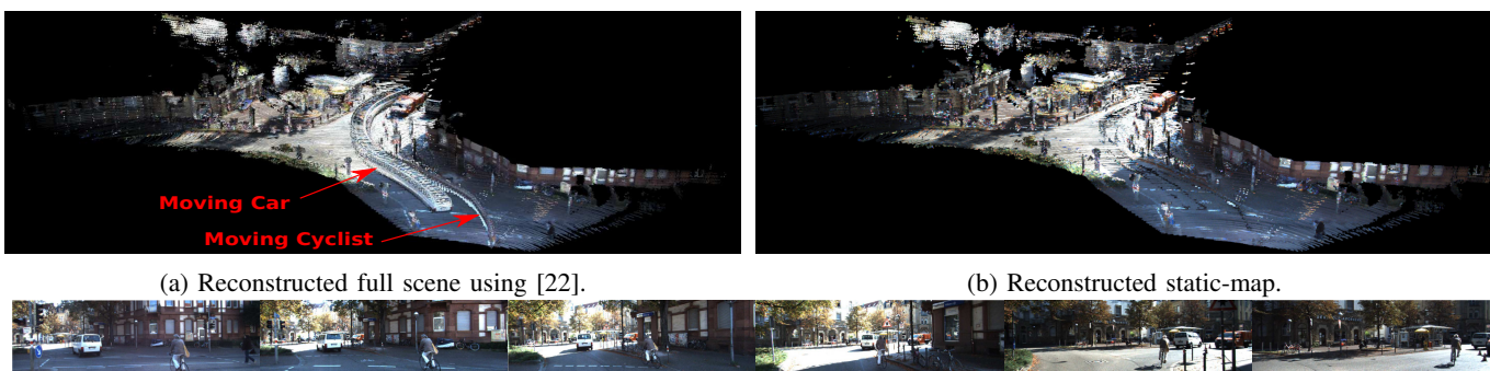
Fig. 6: Junction sequence results: (a) shows the full scene 3D reconstruction using 80 frames. (b) shows the reconstructed static-map without moving objects. Last row images show the corresponding image sequence for every 15 frames.
