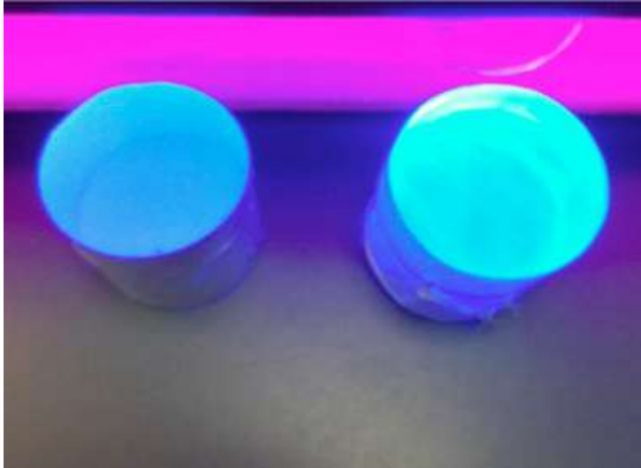
Fig. 4. UV responses of 0.8 wt% bismuth-loaded plastic scintillator (left) and reference EJ-200 (right).
