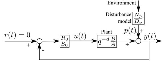
Figure 5. Feedback regulation scheme for rejection of disturbances.
