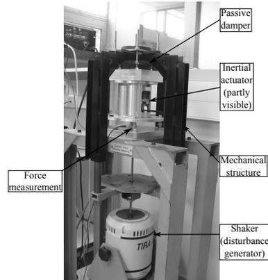
Figure 2. The active vibration control system (photo).
