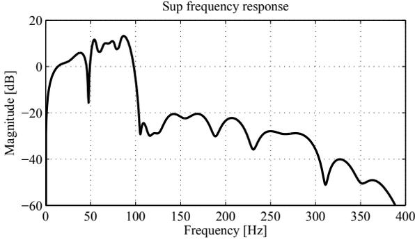
Figure 7. Input sensitivity function with the linear controller.
