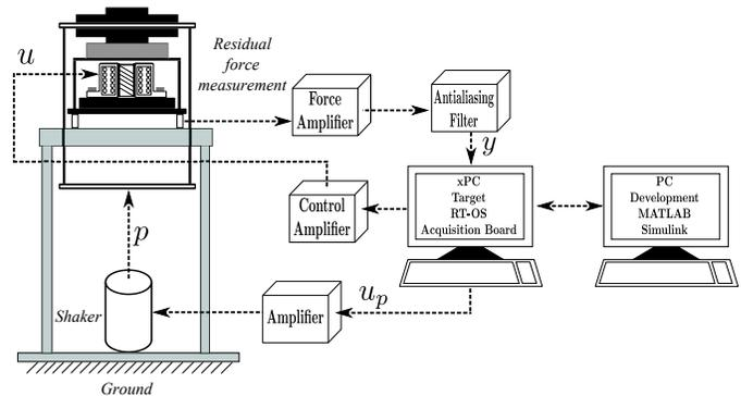
Figure 3. The active vibration control data acquisition diagram.
