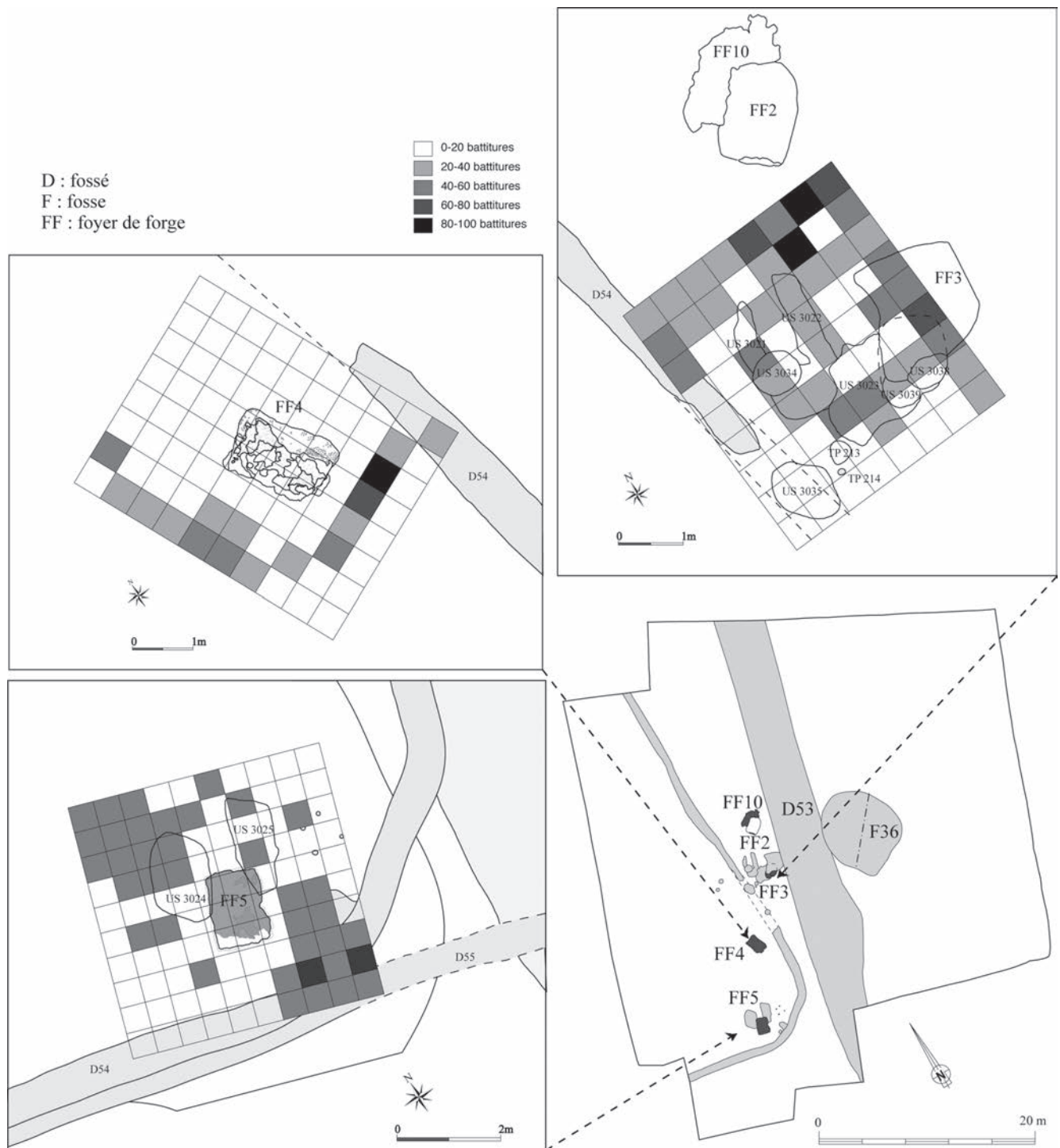
Figure 3 : Plan des structures métallurgiques et répartition des battitures autour des foyers de forge. Figure 3: Plan of the iron working features and hammer scale distribution around the forge hearths.
