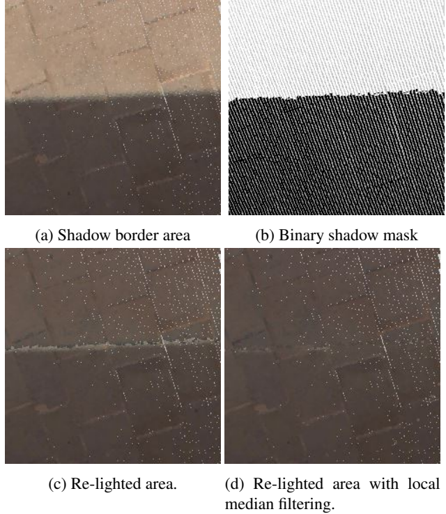
Figure 4: Small penumbra zones on the boundary of a shadow can have non negligible effect when re-lighting a point cloud.
