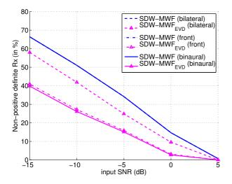
Fig. 2. Percentage of estimated  $R_{\it s}$  's that are not positive definite (SDW-MWF and SDW-MWF  $_{\rm EVD})$
