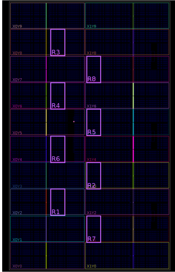
Fig. 4. Example of the result of our floorplanning algorithm (8 regions, 1000 slices, 8 BRAMs, 6 DSPs) on a Virtex7 690t
