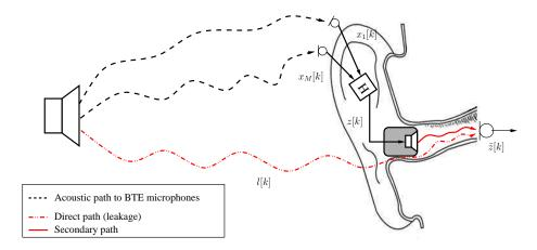
Figure 1: Hearing aid with an open fitting
