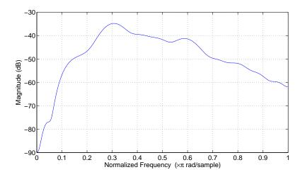
Figure 2: Frequency response of the secondary path filter  $\mathbf{c}[k]$  at 16kHz
