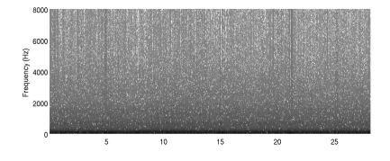
Figure 6: Spectrogram of the car noise signal
