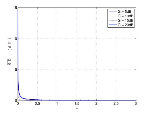
Figure 10: Normalised speech distortion introduced by the weighted integrated ANC and NR scheme (car noise)
