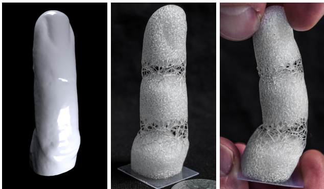
Figure 15: Finger with articulations. Right: deformed object. Note that the inferior articulation is made wider and thus bends further. Model: Olivier hand (AIM@SHAPE Project).
