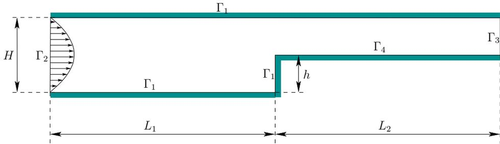
FIGURE 1. Horizontal channel with an abrupt contraction.
