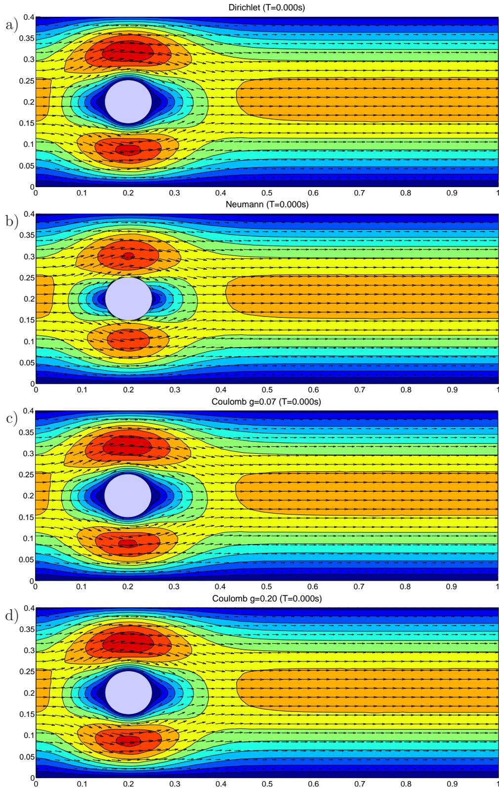
FIGURE 10. Velocity field at  $t = 0$ , obtained as the solution of Stokes equation with different boundary conditions on  $\Gamma_4$  (with  $Re = 100$ ): a) Homogeneous Dirichlet boundary condition b) Neumann boundary condition c) Coulomb boundary condition with  $g = 0.07$  d) Coulomb boundary condition with  $g = 0.20$
