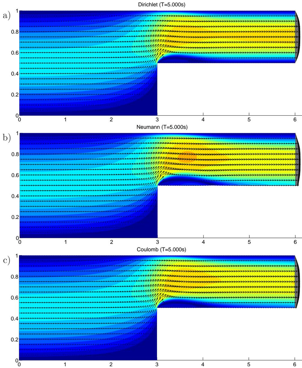
FIGURE 5. Velocity field at  $t = 5s$ , obtained as the solution of Navier–Stokes equation with the three boundary conditions on  $\Gamma_4$ : a) Homogeneous Dirichlet boundary condition; b) Neumann boundary condition; c) Coulomb boundary condition.
