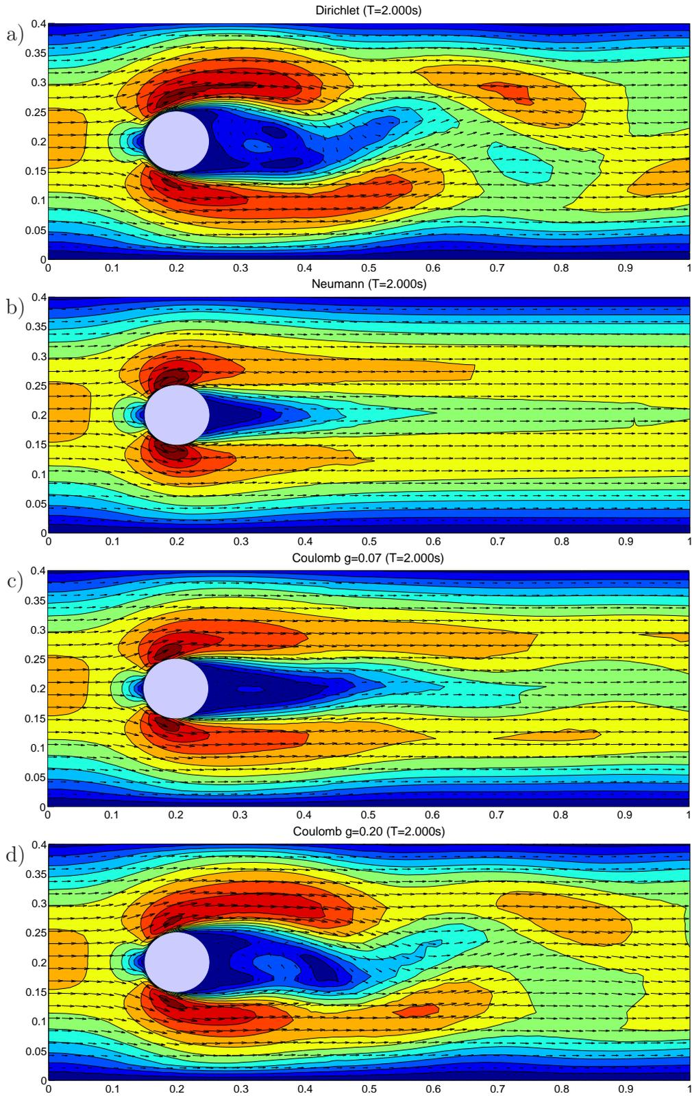
FIGURE 11. Velocity field at  $t = 2s$ , obtained as the solution of Navier-Stokes equation with the four boundary conditions on  $\Gamma_4$  (with  $Re = 100$ ): a) Zero Dirichlet boundary condition b) Neumann boundary condition c) Coulomb boundary condition with  $g = 0.07$  d) Coulomb boundary condition with  $g = 0.20$
