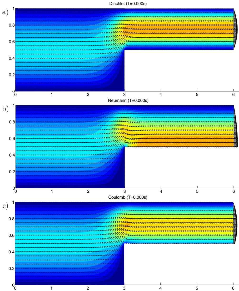
FIGURE 3. Velocity field at  $t = 0$ , obtained as the solution of the Stokes system with the following boundary conditions on  $\Gamma_4$ : a) Homogeneous Dirichlet boundary condition; b) Neumann boundary condition; c) Coulomb boundary condition.
