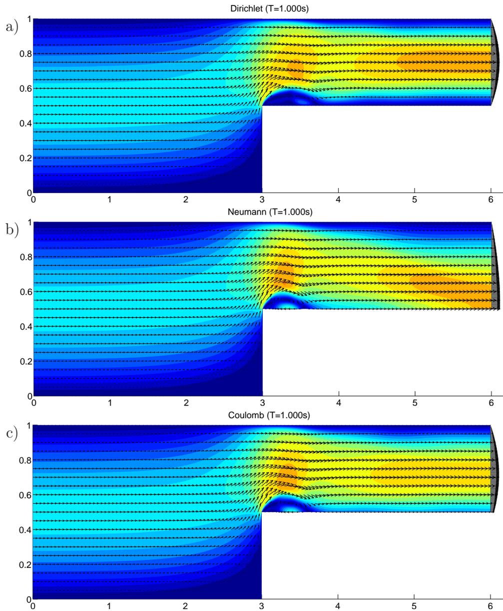
FIGURE 4. Velocity field at  $t = 1s$ , obtained as the solution of Navier–Stokes equation with the three boundary conditions on  $\Gamma_4$ : a) Homogeneous Dirichlet boundary condition; b) Neumann boundary condition; c) Coulomb boundary condition.
