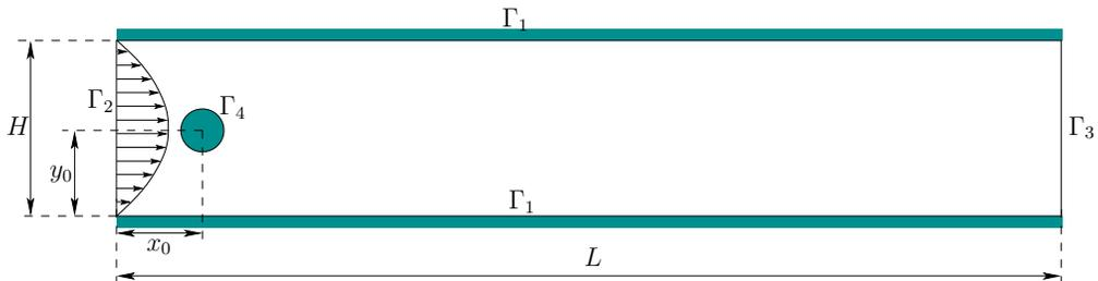
FIGURE 2. Horizontal channel with a cylindrical obstacle.
