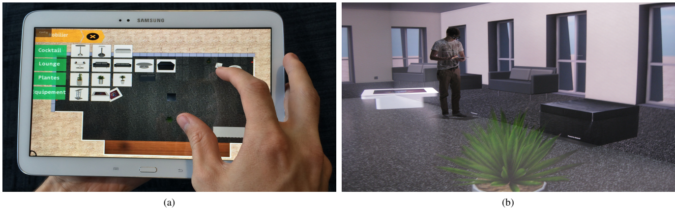
Fig. 4: The redistributed World-In-Miniature: an example of redistribution that demonstrates how it can be used for platform combination. Here the redistribution is performed between a CAVE and a tablet. (a) On the tablet, the user has a plan view of the virtual world at a reduced scale with 2D interaction capabilities. (b) At the same time, the user is immersed at scale one in the same shared virtual world in a CAVE.
