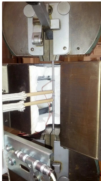
Figure 2: Experimental setup for the tensile tests on single tubes.
