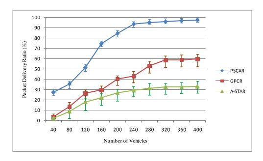
Figure 9: Packet Delivery Ratio over Number of Vehicles.
