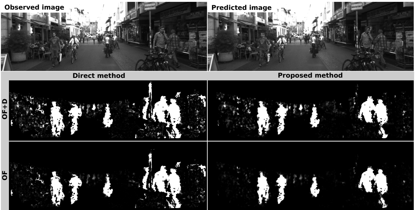
Fig. 11. Several \xi^2(M) images from sequence 09/29-0071, for M = \{\delta u, \delta v, \delta d\} (second row) and M = \{\delta u, \delta v\} (third row) by applying direct approach (left column) and the proposed one (right column). First row shows the observed and the predicted image.
