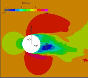
**Fig. 11.** x-component of the dimensionless velocity  $u_x/U_\infty$ , on a cutting plane normal to the cylinder axis. *Left*: instantaneous field. *Right*: filtered field (by adaptive Kalman filter) at the same instant. Results from Run-A. The unit vectors of the coordinate system (x/D, y/D) are shown.
