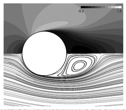
Fig. 6. Time-averaged velocity field from LES (reference simulation: Run-A). Top: Normalized axial velocity  $\langle u_x \rangle / U_\infty$ . Bottom: Two-dimensional streamlines of the mean flow. The grey square on the horizontal axis indicates the downstream end of the recirculation bubble:  $\langle u_x \rangle = 0$  for  $x = \ell_c$  and y = 0;  $\ell_c$  is the wake-closure length.
