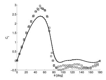
**Fig. 3.** Mean friction coefficient around the cylinder. LES at Re =  $4.7 \cdot 10^4$  (Run-A: solid line, Run-B: dashed line, Run-C: dotted line) are compared with experimental data ( $\square$ : Re =  $10^5$ [33]).
