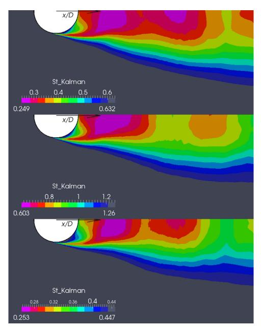
**Fig. 14.** Comparison of the time-averaged *cut-off Strouhal number*  $\langle St_K \rangle$ , between Run-A (top), Run-B (middle) and Run-C (bottom). The unit vectors of the coordinate system (x/D, y/D) are shown.
