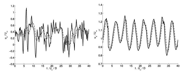
**Fig. 15.** Time records of the dimensionless axial velocity on the centerline of the wake: x/D = 1.7 and y/D = 0 (*Left*) and outside of the wake: x/D = 1.7 and y/D = 1.2 (*Right*), from Run-A. —: instantaneous signal,  $-\cdot-\cdot$ —: filtered signal.
