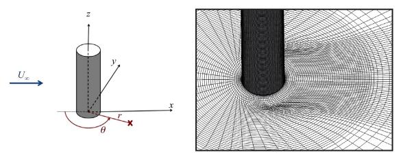
**Fig. 1.** Left: sketch of the Cartesian coordinate system (x, y, z) and the cylindrical coordinate system  $(r, \theta, z)$ . Right: close-up view of the mesh around the cylinder. For clarity, every other point is displayed in each direction.
