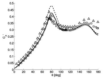
**Fig. 5.** Root-mean-squared pressure coefficient around the cylinder. LES at Re =  $4.7 \cdot 10^4$  (Run-A: solid line, Run-B: dashed line, Run-C: dotted line) are compared with experimental data ( $\square$ : Re =  $6.1 \cdot 10^4$  [36];  $\triangle$ : Re =  $6.1 \cdot 10^4$  [39]).
