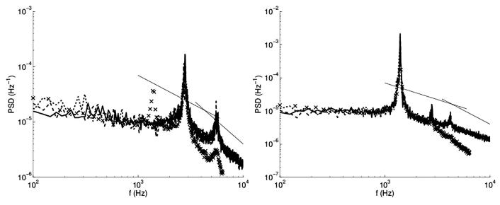
**Fig. 9.** Power spectra of the streamwise velocity  $u_{xy}$  (as measured by a hot-wire anemometer) at x/D = 1.7 and y/D = 0 (*Left*) and y/D = 0.6 (*Right*). Spectra from simulations Run-A: solid line, Run-B: dashed line, Run-C: dotted line. Experimental spectra are indicated by crosses. The characteristic scalings:  $f^{-1}$  (sheared turbulence) and  $f^{-5/3}$  (isotropic turbulence) are shown for indication.
