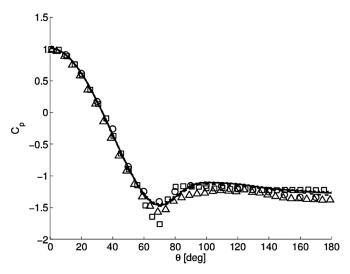
**Fig. 4.** Mean pressure coefficient around the cylinder. LES at Re =  $4.7 \cdot 10^4$  (Run-A: solid line, Run-B: dashed line, Run-C: dotted line) are compared with experimental data ( $\bigcirc$ : Re =  $4.6 \cdot 10^4$  [38],  $\square$ : Re =  $10^5$  [33],  $\triangle$ : Re =  $1.3 \cdot 10^5$  [30]).
