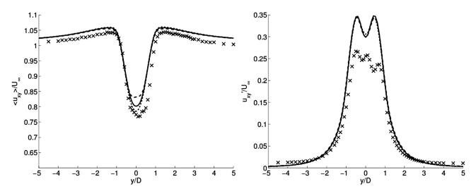
**Fig. 8.** Profiles of the streamwise velocity along the *y*-axis (transverse direction) at position x = 1.7D in the cylinder wake. *Left*: mean velocity. *Right*: root-mean-squared velocity fluctuations. —: LES at Re =  $4.7 \times 10^4$  (Run-A: solid line, Run-B: dashed line, Run-C: dotted line); × : experimental data at Re =  $4.7 \times 10^4$  [41].
