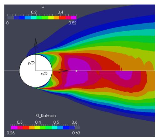
Fig. 13. Upper half: Isocontours of the local turbulence rate defined as  $Tu \equiv \sqrt{(u'^2 + v'^2 + w'^2)/3}/U_{\infty}$ . Lower half: Isocontours of the time-averaged Strouhal number based on the Kalman cut-off frequency:  $\langle St_K \rangle$ . The grey square indicates the end of the mean-recirculation bubble (location of the wake closure). Results from Run-A. The unit vectors of the coordinate system (x/D, y/D) are shown.
