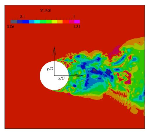
**Fig. 12.** Instantaneous isocontours of the Strouhal number based on the cut-off frequency of the Kalman filter:  $St_K(\mathbf{x},t) = f_{Kalman}(\mathbf{x},t) \cdot D/U_{\infty}$  on a plane normal to the cylinder axis, at the same position and time as in Fig. 11. Results from Run-A. The unit vectors of the coordinate system (x/D, y/D) are shown.
