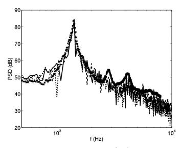
**Fig. 10.** Far-field power spectrum of the pressure (in Pa<sup>2</sup>.Hz<sup>-1</sup>) represented in decibels with reference pressure  $2 \cdot 10^{-5}$  Pa, at position x/D = 15.5 and y/D = 185. Spectra from simulations Run-A: solid line, Run-B: dashed line, Run-C: dotted line. Experimental spectrum is indicated by crosses.
