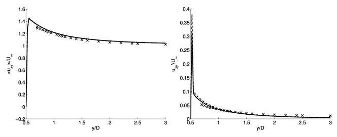
Fig. 7. Profiles of the streamwise velocity along the y-axis (transverse direction) at position x = 0 on one side of the cylinder. Left: mean velocity. Right: root-mean-squared velocity fluctuations. —: LES at  $Re = 4.7 \times 10^4$  (Run-A: solid line, Run-B: dashed line, Run-C: dotted line);  $\times$ : experimental data at  $Re = 4.7 \times 10^4$  [41].
