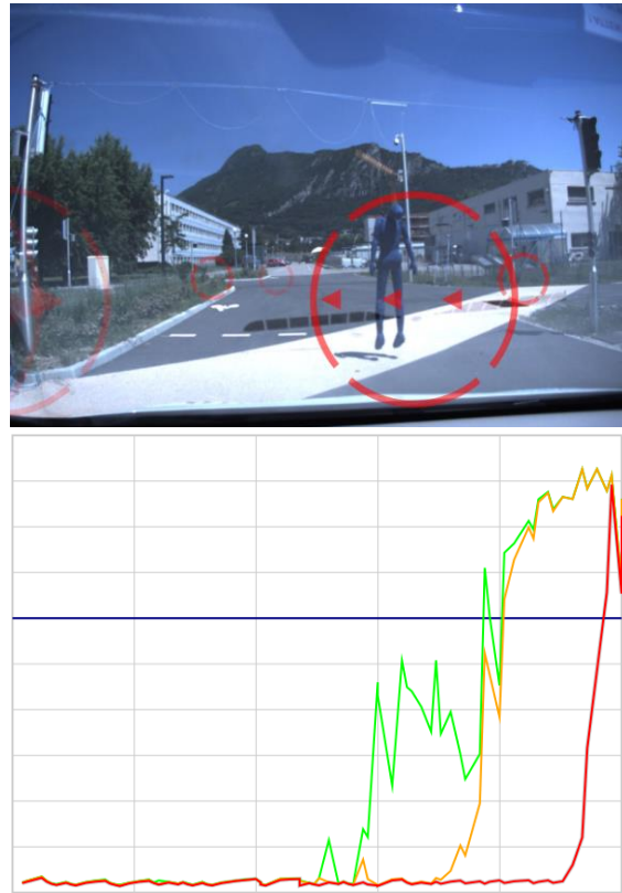
Figure 19: On the upper camera image, red circles correspond to collision risks and arrows the direction of moving targets. On the lower image, graphs correspond to collision risk probabilities for 3 time horizons: 1s (red), 2s (yellow) and 3s (green).
