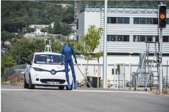
Figure 17: Risk collision experiments with our dummy crossing a street. © Inria / Photo H. Raguét.
