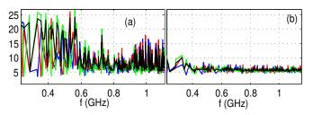
Fig. 4. Electric field localization index (dB), (a) in the classical RC, (b) in the chaotic cavity (blue for x-, red for y- and green for z-component and black for  ${\bf L}_{tot}^E$ ).
