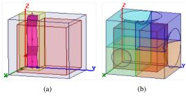
Fig. 5. Integration volumes (a) within the classical RC: volumes  $V_b$  and  $V_z$ , and (b) within the chaotic cavity: peripheral volumes  $(V_1, V_2, V_3, V_4)$  and central volume  $V_c$ .
