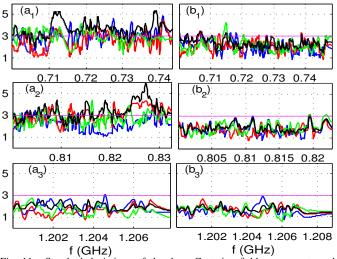
Fig. 11. Standard deviations of the three Cartesian field components and total one (blue for  $\sigma_x$ , red for  $\sigma_y$ , green for  $\sigma_z$ , and black for  $\sigma_{tot}$ ) for  $(a_1, a_2, a_3)$  cavity  $C_1$  and  $(b_1, b_2, b_3)$  cavity  $C_2$  in the three frequency bands for a source located in  $(S_1)$ .
