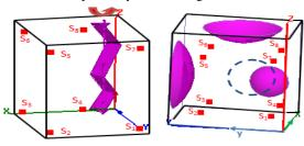
(a) Classical RC (C1) (b) Chaotic cavity (C2) Fig. 3. Chaotic and classical cavities with 8 points sources  $S_i$ .
