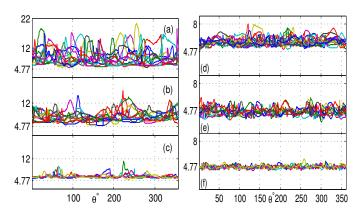
Fig. 8. Global  $L^E_{tot}$  (in dB) versus stirrer/hemisphere position (whole rotation with  $1^\circ$  step) in conventional (a-c) and chaotic (d-f) cavities, (a)&(d) 15 modes above 700 MHz, (b)&(e) 10 modes above 800 MHz and (c)&(f) 6 modes above 1.2 GHz.
