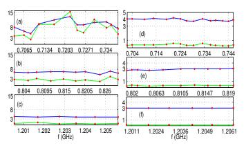
Fig. 9. Means (blue) and standard deviations (green) over stirrer/hemisphere rotation of the global  $L^E_{tot}$  (linear scale), in conventional (a-c) and chaotic (d-f) cavities, (a)&(d) 15 modes above 700 MHz, (b)&(e) 10 modes above 800 MHz and (c)&(f) 6 modes above 1.2 GHz. The values for each mode are indicated at its resonant frequency at the initial stirrer/hemisphere position.
