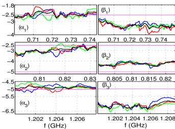
Fig. 12. Amplitude of the field anisotropy coefficients (in dB) versus frequency (blue for  $A_{xy}$ , red for  $A_{yz}$ , green for  $A_{zx}$ , and black for  $A_{tot}$ ) for  $(\alpha_1,\alpha_2,\alpha_3)$  cavity  $C_1$  and  $(\beta_1,\beta_2,\beta_3)$  cavity  $C_2$ , source location  $(S_1)$  in the three frequency bands.
