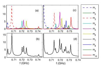
Fig. 10. Amplitude of the modal contribution  $|E_{m(\omega)}|$  at the center of working volume for the eigenmodes  $m_i$  ((a) for classical cavity and (c) for chaotic cavity); and amplitude of the total electric field induced by their contribution ((b) for classical cavity and (d) for chaotic cavity).
