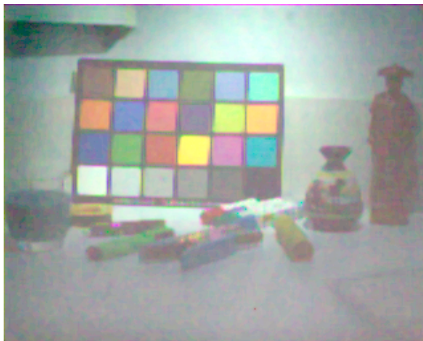
Figure 13. sRGB image of scene 1 computed according to a colorimetric calibration of the sensor. Color image is provided as Supplementary Materials in Figure S5.
