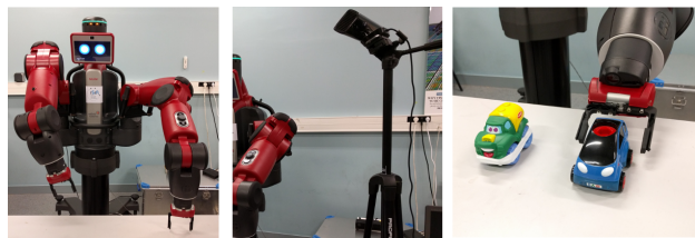
Fig. 4. Experiment setup. Baxter robotics platform (left). Kinect sensor (middle). Subset of objects of interest (right).
