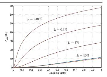
**Figure 7.** Attenuation  $A_{\rm dB}$  achievable with the four shunt layouts as a function of the coupling factor  $k_i$  (for the R-shunt) and of the enhanced coupling factor  $\tilde{k}_i$  for the shunts with NC (parallel, series and SP), for several values of structural damping  $\xi_i$ . For each value of  $\xi_i$ , four curves are merged, one for each configuration: parallel, series, SP and simple resistive shunt.
