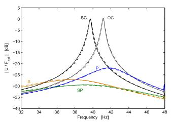
Figure 22. FRFs (displacement U to force  $F_{\rm ext}$  ratio), around the first resonance of the EMS, for different configurations, analogous to figure 4. Comparison of experiments (solid lines) and theory (dashed lines).
