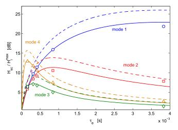
Figure 20. The trend of  $H_{\rm sc}/H_i^{\rm max}$  as a function of  $au_e$  for the parallel configuration, for the four modes of the experimental set-up. The solid lines are related to the analytical model using  $C_{pi}$  (equations (8) and (9)), the dashed lines to the analytical model using  $C_{\infty}$ (equation (6)), and the markers to experiments ( $\circ$ : mode 1;  $\square$ : mode 2; ' $\Diamond$ ': mode 3; ' $\triangle$ ': mode 4).
