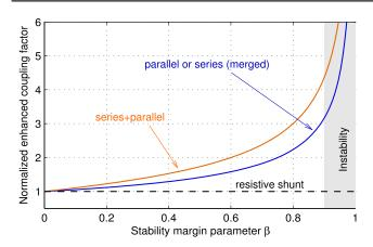
**Figure 6.** The trend of the EMEMCF  $\tilde{k}_i$ , normalised by  $k_i$  ( $\tilde{k}_i/k_i$ ), as a function of  $\beta$ , for the three NC configurations (parallel, series and series+parallel), with  $\beta = \beta_p = \beta_s = \beta_{sp1} = \beta_{sp2}$ . The grey region shows an example of the region for which the system is unstable, for  $\beta$  above 0.9 in this particular case.
