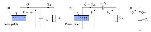
Figure 3. Shunt with the addition of an NC: (a) parallel configuration; (b) series configuration. (c) Definition of an NC.
