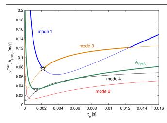
**Figure 9.** The trend of  $v_i^{\text{max}}$  and  $A_{\text{RMS}}$  for the four modes of the EMS described in table 5 for an NC in series configuration.  $C_{\text{p}i} = 30.5 \text{ nF}$  and  $C_2 = 36.6 \text{ nF}$ . The values of the mode shape components used here are:  $\Phi(x_f) = [1.7167, 0.2450, 0.8020, 1.1987]'$  and  $\Phi(x_m) = [2.3452, 2.2935, -2.8761, -2.2822]'$ .
