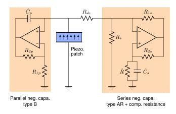
Figure 14. Electronic circuit used for the SP configuration.
