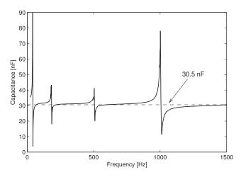
**Figure 16.** Experimental capacitance  $C(\Omega)$  as a function of frequency of the piezoelectric patches in series.
