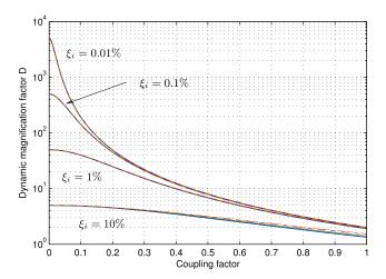
**Figure 8.** The magnification factor at resonance D due to the four shunt layouts as a function of the coupling factor  $k_i$  (for the R-shunt) and of the enhanced coupling factor  $\tilde{k}_i$  for the shunts with NC (parallel, series and SP), for several values of structural damping  $\xi_i$ . For each value of  $\xi_i$ , four curves are merged, one for each configuration: parallel, series, SP and simple resistive shunt.
