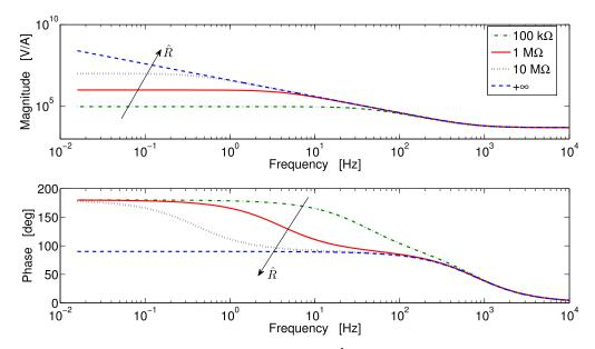
Figure 13. Magnitude and phase of the impedance  $Z_{rs}$  for different values of  $\hat{R}$ . In this figure:  $R_1 = R_2 = 5 \text{ k}\Omega$ ,  $R_{sh} = 50 \text{ k}\Omega$  and  $\hat{C} = 40 \text{ nF}$ . The case with  $\hat{R} = +\infty$  corresponds to an IC (i.e.  $Z_{is}$ ).
