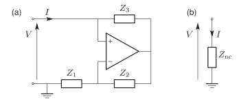
Figure 10. A negative impedance built by means of an OP-AMP (a) and its electrical model (b).
