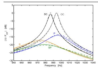
**Figure 23.** FRFs (displacement U to force  $F_{\rm ext}$  ratio), around the fourth resonance of the EMS, for different configurations, analogous to figure 4. Comparison of experiments (solid lines) and theory (dashed lines).
