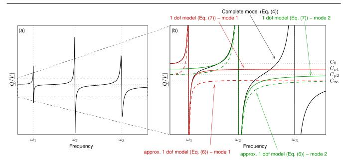
**Figure 2.** The trend of  $C(\omega) = |\underline{Q}/\underline{V}|$  for a generic, undamped three-degrees-of-freedom system. (a) The complete model of equation (4); (b) zoom showing the complete model (black) of equation (4) and the 1 dof models of equation (6) (dashed lines) and (7) (solid lines) tuned to mode 1 (red) and mode 2 (green). Note that the continuous lines relating to equations (4) and (7) (red line, first mode) are fully superimposed before  $\omega_1$ .
