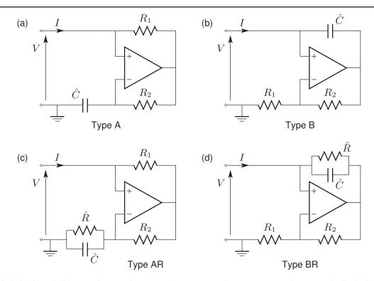
**Figure 11.** Practical circuits to build a negative capacitance: type A (a), type B (b), type AR (c) and type BR (d) circuits in parallel configuration. For the series configuration, the pins of the OP-AMP must be exchanged.
