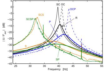
**Figure 21.** Experimental FRFs (displacement U to force  $F_{\text{ext}}$  ratio), around the first resonance of the EMS, for different configurations, analogous to figure 4 (except for the short circuit response of the SP configuration (SCSP) that is slightly distinct to SCS in experiments).
