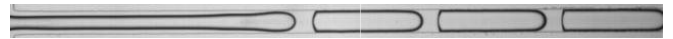
Video 8. Movie illustrating the monodisperse fragmentation of the thread under synchronised chopped laser forcing ( f \simeq f^* ). The real-time dynamics is ten times faster; P = 31 mW, f = 12 Hz, (Q_w, Q_o) = (2, 1) \mu\text{L min}^{-1} .
