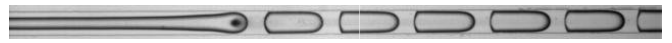
Video 6. Movie illustrating the monodisperse fragmentation (1 drop every 2 periods) of the thread under chopped laser forcing. The real-time dynamics is twenty times faster; P = 67 mW, f = 50 Hz, (Q_w, Q_o) = (2, 1) \mu\text{L min}^{-1} .
