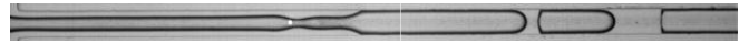
Video 5. Movie illustrating the low-frequency ( f < f^* ) multi-disperse fragmentation of the thread under chopped laser forcing. The real-time dynamics is ten times faster; P = 37 mW, f = 5 Hz, (Q_w, Q_o) = (2, 1) \mu\text{L min}^{-1} .
