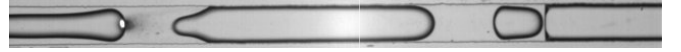
Video 4. Movie illustrating the high-periodic (here, period-4) fragmentation of the thread under continuous laser forcing. The thread interface alternatively does and does not touch the lateral walls. The real-time dynamics is ten times faster; P = 45 mW, (Q_w, Q_o) = (2, 1) \mu\text{L min}^{-1} .
