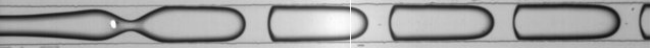
Video 2. Movie illustrating the permanent fragmentation of the thread in the stationary fragmented regime. The thread interface never touches the lateral walls. The real-time dynamics is ten times faster; P = 37 mW, (Q_w, Q_o) = (2, 1) \mu\text{L min}^{-1} .
