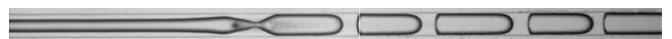
Video 7. Movie illustrating the high-frequency ( f > f^* ) multi-disperse fragmentation of the thread under chopped laser forcing (1 drop in 2 and 3 periods in alternation). The real-time dynamics is twenty times faster; P = 55 mW, f = 50 Hz, (Q_w, Q_o) = (2, 1) \mu\text{L min}^{-1} .
