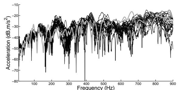
**Fig. 6** Observation 2: experimental FRF measurements (black lines), deterministic FRF using the C-NROM (gray line)
