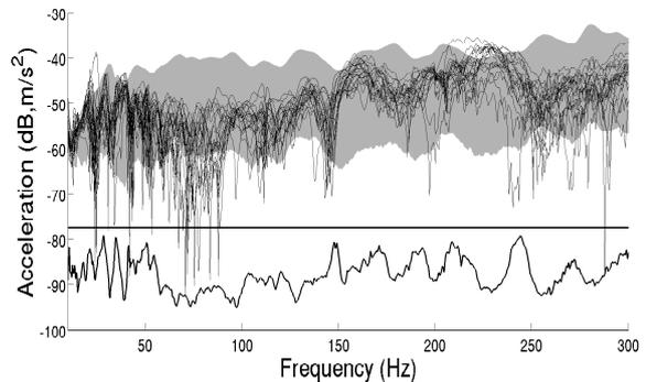
**Fig. 21** Observation 1, zoom into band  $\mathcal{B}_L \cup \mathcal{B}_M$ : experimental FRF measurements (black lines), random FRF using the identified ML-SROM (gray region), and OVL function (black line underneath)
