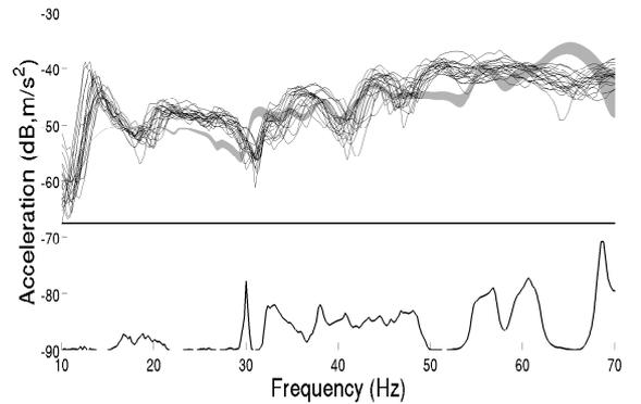
**Fig. 14** Observation 2, zoom into band  $\mathcal{B}_L$ : experimental FRF measurements (black lines), random FRF using the identified C-SROM (gray region), and overlap function OVL (black line underneath)
