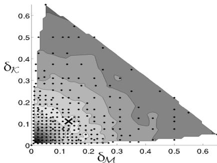
**Fig. 7** Plot of function  $(\delta_{\mathcal{M}}, \delta_{\mathcal{K}}) \mapsto J_s(\delta_{\mathcal{M}}, \delta_{\mathcal{K}})$  for the identification of hyperparameters  $\delta_{\mathcal{M}}$  and  $\delta_{\mathcal{K}}$  of the C-SROM. Black dots: sampling points, black cross: optimal point.
