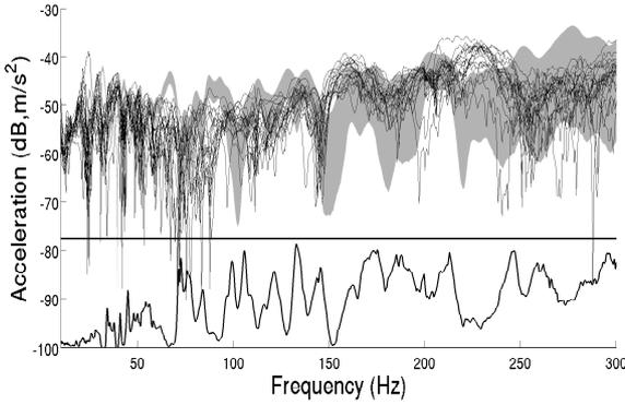
**Fig. 11** Observation 1, zoom into band  $\mathcal{B}_L \cup \mathcal{B}_M$ : experimental FRF measurements (black lines), random FRF using the identified C-SROM (gray region), and overlap function OVL (black line underneath)
