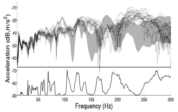
**Fig. 12** Observation 2, zoom into band  $\mathcal{B}_L \cup \mathcal{B}_M$ : experimental FRF measurements (black lines), random FRF using the identified C-SROM (gray region), and overlap function OVL (black line underneath)
