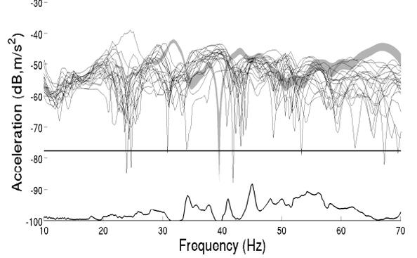
**Fig. 13** Observation 1, zoom into band  $\mathcal{B}_L$ : experimental FRF measurements (black lines), random FRF using the identified C-SROM (gray region), and overlap function OVL (black line underneath)
