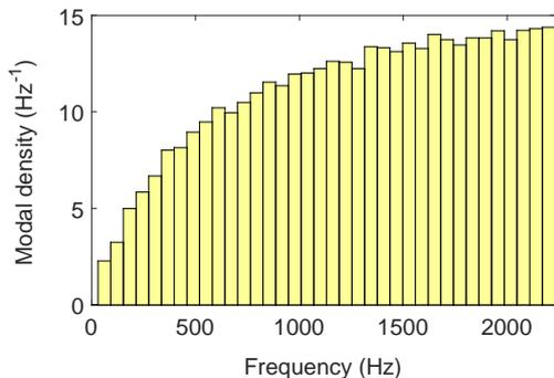
**Fig. 2** Modal density calculated with the computational model.
