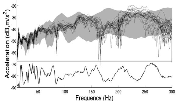
**Fig. 22** Observation 2, zoom into band  $\mathcal{B}_L \cup \mathcal{B}_M$ : experimental FRF measurements (black lines), random FRF using the identified ML-SROM (gray region), and OVL function (black line underneath)
