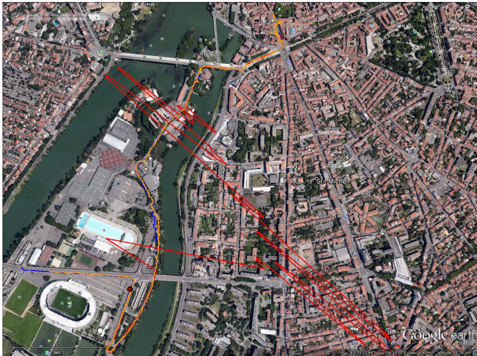
Fig. 8. Position given by a noiseless GPS receiver (color orange), by a faulty GPS receiver when B_{PLL} = 4Hz, B_{FLL} = 4Hz, p = 0.1 (color red), a faulty GPS receiver when B_{PLL} = 12Hz, B_{FLL} = 4Hz, p = 0.3 (color blue) displayed using Google earth
