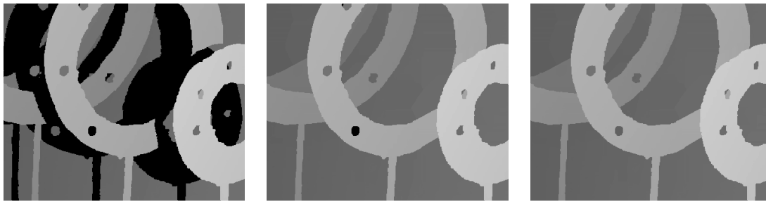
Fig. 7. Inpainting of rings. Left: synthesized depth-map with the holes in black. Middle: result after the line extension and diffusion process. Right: final result after inpainting the remaining holes.
