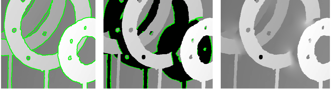
Fig. 4. Left: exterior narrow band NB_o^+ superimposed on the original depth-map J_o . Middle: exterior narrow band NB_s^+ superimposed on the synthesized depth-map J_s . Inpainting result with [13] while taking the exterior narrow band NB_s^+ (middle) as source for the diffusion. See text for details.
