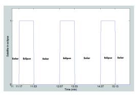
Fig. 1: The analysis is for 24 hours but for clarity of presentation only a few hours are depicted. This satellite performs a full circle around the earth around 14 times over 24h, with average cycle duration of around 100 minutes. Out of the 100 minute cycle, around 36 minutes are spent in the earth's umbra.
