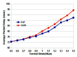
Fig. 3: As expected, with SLIM there is a slight increase in end-to-end delay. The bigger gap for higher load is in part due to the fact that, as shown in Fig. 4(b), for these values the network is congested and SLIM delivers more packets than DSP.
