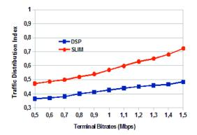
(a) Load Distribution Index for different terminal bitrates
