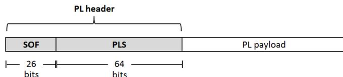
Fig. 1: PL frame structure
