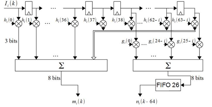
Fig. 8: Hardware implementation of  $G_i$  and  $H_i$  filters using SR and FIFO for real part
