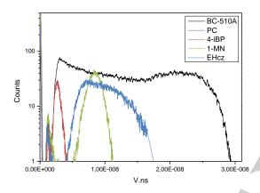
**Figure 5**. Comparison of the <sup>137</sup>Cs scintillation gamma spectra obtained for BC-501A (black), *N*-(2-ethylhexyl)carbazole (blue), 1-methylnaphthalene (green), 4-isopropylbiphenyl (red), where the background residual signal has been discarded. Data were obtained for 3 mL liquid samples.
