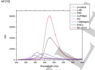
**Figure 3.** Radioluminescence spectra of pure liquids under β irradiation ( $^{90}$ Sr- $^{90}$ Y – 36 MBq): *p*-xylene, LAB, DIN, 4-isopropylbiphenyl, pseudocumene, 1-methylnaphthalene, BC-501A, and EHCz (from lower to higher wavelengths of maximum emission).
