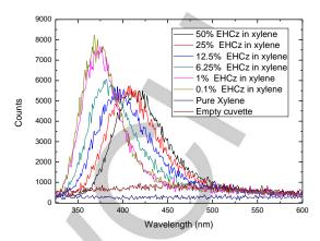
Figure 4. Radioluminescence spectra under  $\beta$  irradiation ( $^{90}Sr^{-90}Y-25$  MBq) for 0 - 50 vol% EHCz in xylene. No emission of xylene is visible in this experiment.
