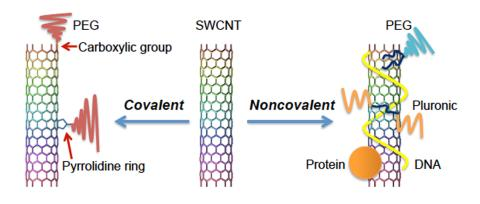
**Figure 3.** Surface modification of SWCNTs for bio-applications. Covalent approaches frequently consist in grafting moieties from pyrrolidine rings or carboxylic groups while noncovalent approaches are based on SWCNTs encapsulation using amphiphilic molecules. Examples of PEG (e.g. PL-PEG), pluronic (e.g. F108), proteins (e.g. BSA) and single-strand DNA are pictured.
