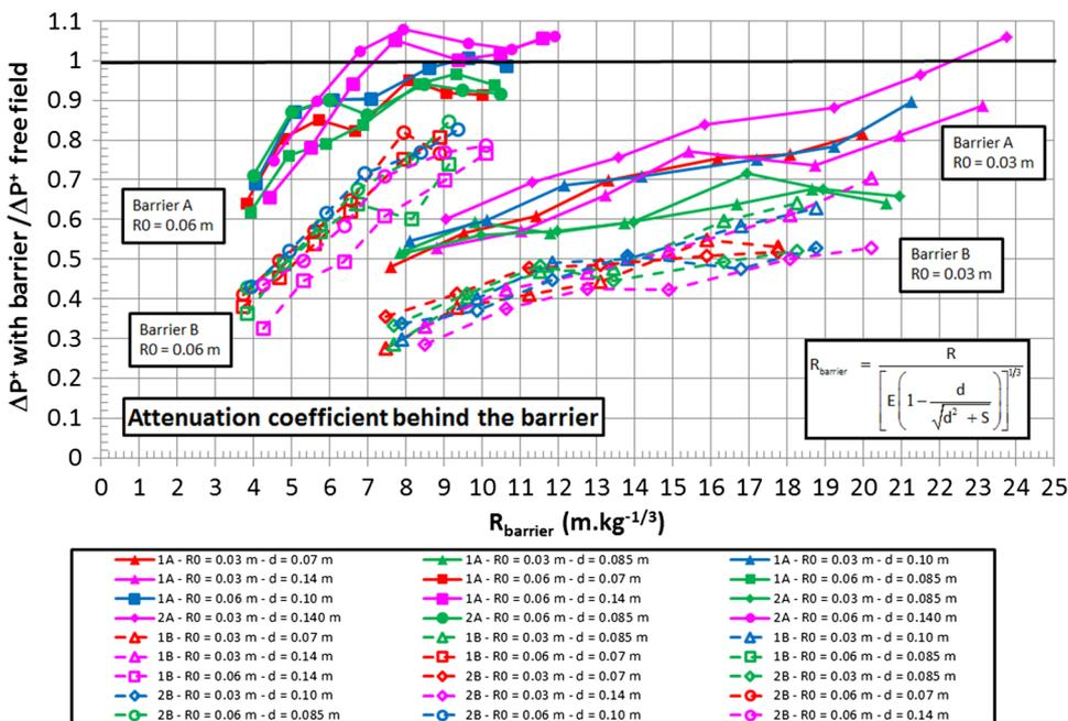
**Fig. 12** Evolution of the attenuation factor downstream from barrier used by Allain [2] for different masses of TNT and distances from the charge to the foot of the barrier
