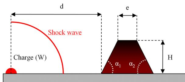
**Fig. 1** Schematic diagram of a protection barrier— $W$  charge mass (kg of TNT),  $d$  distance between centre of charge and the front face (m),  $e$  thickness at crest of obstacle (m),  $H$  height of barrier (m),  $\alpha_1$  angle of inclination of front face ( $^\circ$ ),  $\alpha_2$  angle of inclination of rear face ( $^\circ$ )
