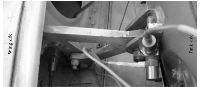
Fig. 7 Instrumentation of the rear attachment of the right wing.
