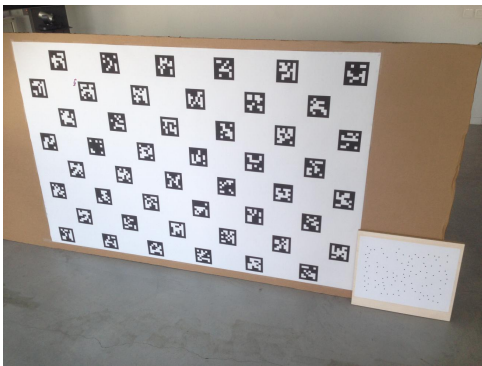
Figure 4: Comparison of a 2 \times A0 calibration board used by Audet's method [1] and a B4 calibration board used by our method (bottom-right) for large focus distances.
