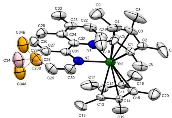
**Figure 7.** ORTEP for the brown crystal obtained from toluene in the thermal reaction of Cp\*<sub>2</sub>Yb(4,7-Me<sub>2</sub>phen), **2** (thermal ellipsoids are at 50% level) and referred to as "compound" **7**. The carbon atoms represented in orange are due to a positional disorder of a methyl group connected to the phenanthroline ring and the carbon atom represented in pink is due to the methylene group.
