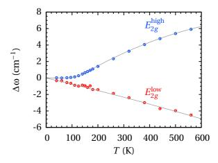
FIG. 5. Calculated frequency shift of the  $E_{2g}$  modes as a function of temperature as obtained by a DFT approach using the experimental lattice parameters determined in Ref. ([25]) and the thermal expansion coefficients reported for temperatures above RT in Ref. ([28]).
