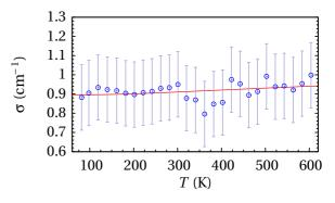
FIG. 7. Temperature dependence of the root-mean-squared width of the Gaussian line shape fitted to the  $E_{2g}^{\rm low}$  Raman peak (empty circles). The solid line is the fit of the anharmonic model taking into account the upconversion process.
