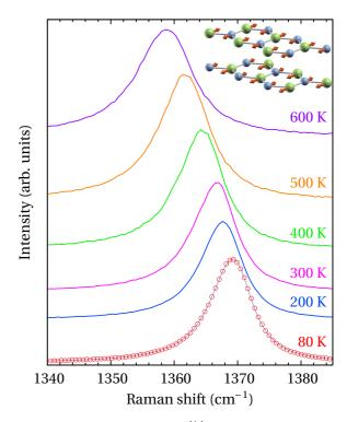
FIG. 3. Raman spectra of the  $E_{2g}^{\rm high}$  mode obtained at different temperatures in backscattering from a c face. Inset, schematic representation of atomic motion for the  $E_{2g}^{\rm high}$  mode.
