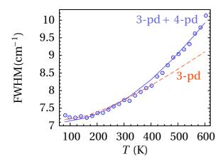
FIG. 6. Temperature dependence of the intrinsic FWHM of the  $E_{2g}^{\rm high}$  mode obtained from the Raman spectra (empty circles). The dashed line is the temperature dependence predicted by the anharmonic model considering only three-phonon decay processes. The solid line is the fit of the anharmonic model taking into account also four-phonon decay processes.
