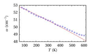
FIG. 8. Temperature dependence of the  $E_{2g}^{\rm low}$  Raman peak frequency (empty circles). The solid line is the temperature dependence calculated from the thermal expansion of the interlayer distance.
