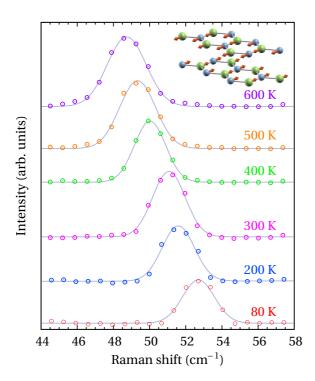
FIG. 4. Raman spectra (empty circles) of the  $E_{2g}^{\text{low}}$  mode obtained at different temperatures in backscattering from a c face. The solid lines correspond to Gaussian line-shape fits to the spectra. Inset, schematic representation of atomic motion for the  $E_{2g}^{\text{low}}$  mode.
