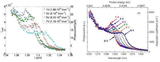
Fig. 2. QCSE in the O-band telecommunication wavelength, based on (a) strain envineering, (b) thickness engineering of the QW structures
