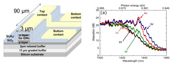
Fig. 1. (a) Schematic view of a Ge/SiGe QW structure in a waveguide configuration that can be used as a modulator or as photodetector. (b) absorption spectra as a function of the applied voltage on the modulator.
