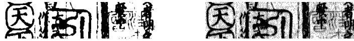
Figure 4: Comparison of thresholding and error diffusion binarization techniques. Left: with thresholding, right: with error diffusion.
